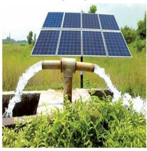
A solar-powered water pump is a pump running on electricity generated by photovoltaic panels or the radiated thermal energy available from collected sunlight as opposed to grid electricity or diesel run water pumps.
